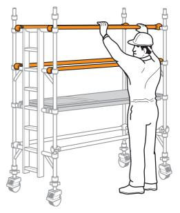
**3** Fit two diagonal braces in opposing directions between the 1<sup>st</sup> and 3<sup>rd</sup> rungs. Ensure that the frames are vertical and level by checking with a spirit level and setting the adjustable legs as necessary. Fit stabilisers (see notes on **page 9**). Fit the next pair of end frames and check the frame interlock clips are engaged.
