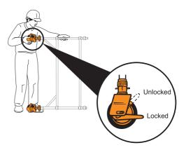
**2** Fit one horizontal brace (red) onto the vertical of a span frame, just above the bottom rung, with the claw facing outwards. The frame will now be self-supporting.
