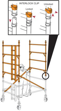
**5** Fit a temporary deck on the lowest rungs. Fit a trapdoor deck on the 4<sup>th</sup> rung (2.0m) with the trapdoor next to the ladder. Ensure the trapdoor is positioned with the hinges towards the outside of the tower as shown. Climb the ladder and, from the protected trapdoor position, fit guardrails on the 5<sup>th</sup> and 6<sup>th</sup> rungs (in that order) on both sides of the platform.
