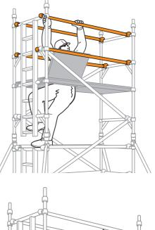
6 Continue the procedure until the required working height is reached, adding additional pairs of end frames, diagonal braces and fitting trapdoor platforms, as shown on previous steps. At every platform level, add horizontal braces as guardrails from the protected position within the trapdoor (as shown in **Step 5**).
