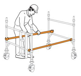
**4** Fit two additional end frames, ensuring the frame interlock clips are engaged. Fit two diagonal braces (blue) in opposing directions, between the 1<sup>st</sup> and the 3<sup>rd</sup> rungs. Ensure the frames are vertical and level by checking with a spirit level and setting the adjustable legs as required.
