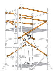
Continue to add pairs of end frames, diagonal braces and fit trapdoor decks as shown in the previous steps. Add guardrails at 0.5m and 1.0m, (in that order), above the platform from the protected trapdoor position.
